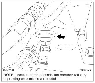
Fig. 2, Transmission Breather (Eaton Fuller shown)
