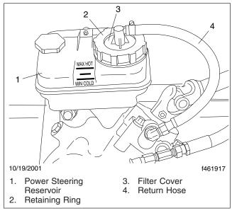
Fig. 1, Power Steering Reservoir
