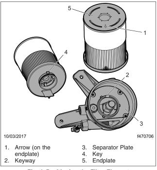
Fig. 4, Positioning the Filter Element
