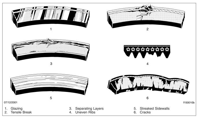
Fig. 1, Drive Belt Replacement Conditions
