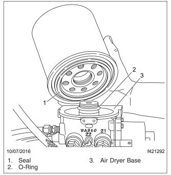
Fig. 9, Desiccant Cartridge Replacement
