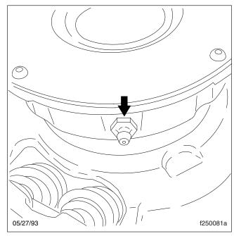
Fig. 1, Release Bearing Grease Fitting
