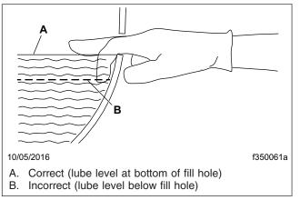
Fig. 3, Axle Lubricant Level Inspection
