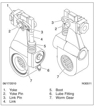
Fig. 5, Bendix Automatic Slack Adjuster
