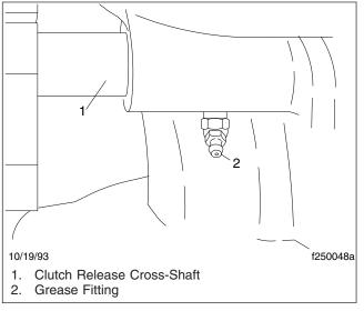
Fig. 3, Cross-Shaft Grease Fitting, Left Side
