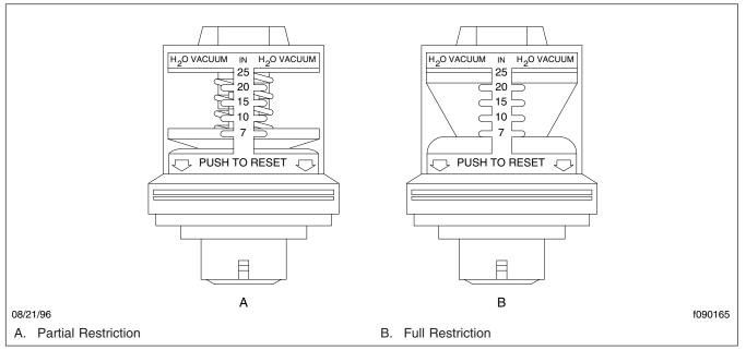
Fig. 1, Air Restriction Indicator, Diesel Engines
