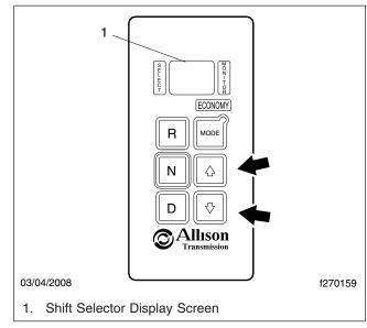
Fig. 6, Transmission Shift Selector
