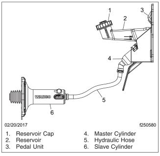
Fig. 5, Clutch Components
