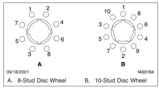
Fig. 1, Wheel Nut Tightening Sequence
