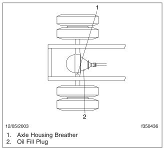
Fig. 2, Component Locations, Meritor Axles
