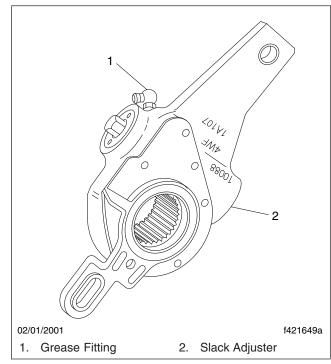
Fig. 3, Haldex Slack Adjuster Grease Fitting
