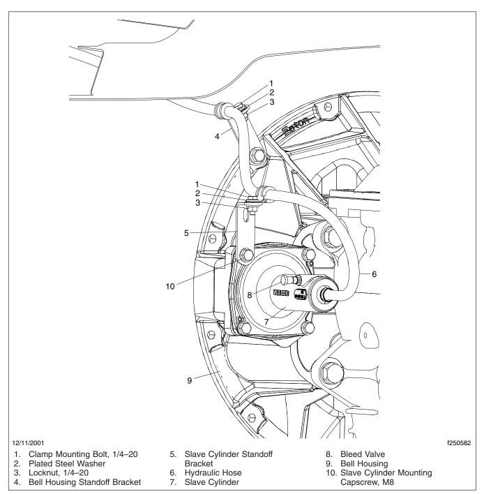
Fig. 6, Clutch Slave Cylinder
