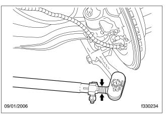
Fig. 4, Checking Tie Rod End Movement
