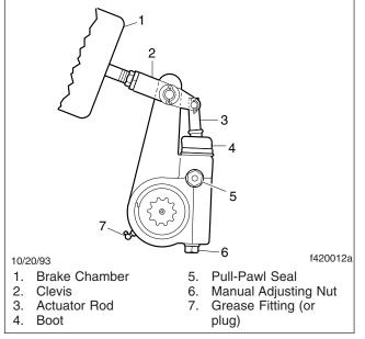
Fig. 4, Meritor Automatic Slack Adjuster
