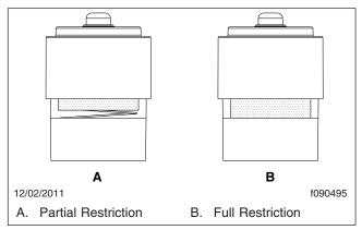
Fig. 2, Air Restriction Indicator, Propane Engines
