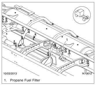
Fig. 7, Fuel Filter Location (fuel going in the engine)
