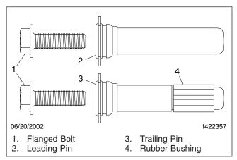
Fig. 8, ZOH-T Slide Pins and Bolts
