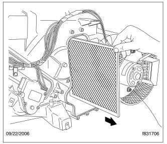
Fig. 2, HVAC Assembly Filter Removal
