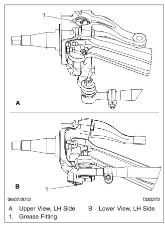
Fig. 1, Grease Fittings, Detroit Axles
