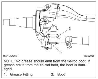
Fig. 5, Grease Fitting and Boot (Detroit axle shown)
