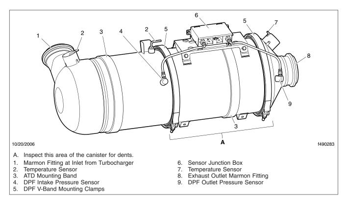
Fig. 2, Typical Aftertreatment Device
