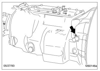
Fig. 4, Cross-Shaft Grease Fitting, Right Side
