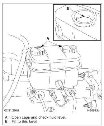
Fig. 7, Hydraulic Brake Fluid Reservoir
