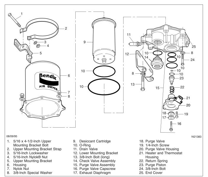
Fig. 1, AD-9 Air Dryer
